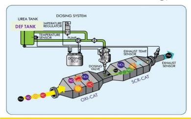
SCR technology uses ammonia to reduce NOx to elemental nitrogen and water.
