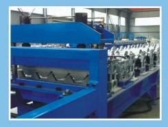
Floor decking roll forming machine is manually used tom produce steel floor decking and can produce high quality floor decking has advantages, such as no cutting deformation, high strength and a large working load. It can be directly mixed with the wielded steel mesh and concrete with good adhesion, Applied in High-rise steel building, it can save the steel molding templates, and also reduce the floor load. Under the same capacity, it can reduce the amount of steel to achieve cost-saving.
