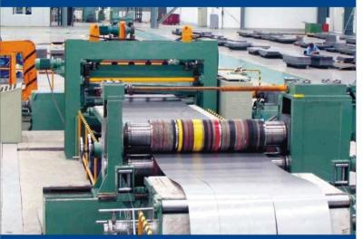
This line can be adjusted to do recoiling or dividing work to meet customers' demands. PLC system is used to select the information from every part of the line, centrally controlled. There also has speed self adjusted and keep memory after lost power supply function. So the line has efficient performance.
