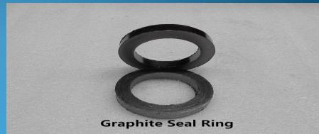
Expanded Graphite yarn reinforced with and without Inconel wire with corrosion inhibitor and thermo Lube Dispersion Ideal for Superheated Saturated steam, Hydrocarbon , chemical valves *Temperature*: -240°C to 650°C *Pressure: 500 Bar Pressure without inconel / SS wire : 80kgF pH: 0 to 14* Applications Valves
