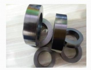
Flexible Graphite Piston Seal Ring. Alternative layers of metallic flexible graphite molded into single ring. For Piston Valves, Safety Valves and High Pressure Valves Temperature : -200 to 650 Deg C
