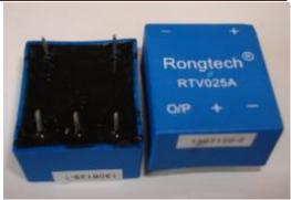
The RTV5, 10/25A series current mode voltage sensor is a device based on the principle of the hall effect, with a galvanic isolation between primary and secondary circuit, It provides accurate electronic measurement of DC AC or pulsed currents.
