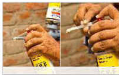
After use, clean the valve & tube immediately with Gun & Foam Cleaner.
