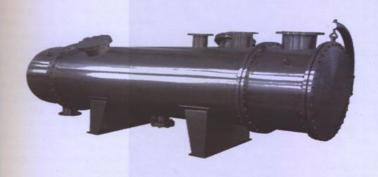
When gas is having design pressure more than 50 bar, then it is recommended to design the Heat Exchanger with Gas on Tube Side & water on shell side. It is a removable tube bundle, outside packed floating tube sheet design
