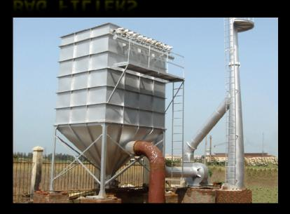
A dust collector is a system used to enhance the quality of air released from industrial and commercial processes by collecting dust and other impurities from air or gas. Designed to handle high-volume dust loads, a dust collector system consists of a blower, dust filter, a filter-cleaning system, and a dust receptacle or dust removal system. It is distinguished from air cleaners, which use disposable filters to remove dust.
