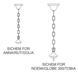
ALL THE HEADS EXCEPTING GLOBE 250 AND GLOBE 300 CAN BE FITTED UPWARDS OR DOWNWARDS
