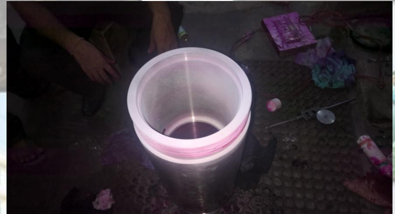
Visible Dye Penetrant Testing of Forged/Machined item
