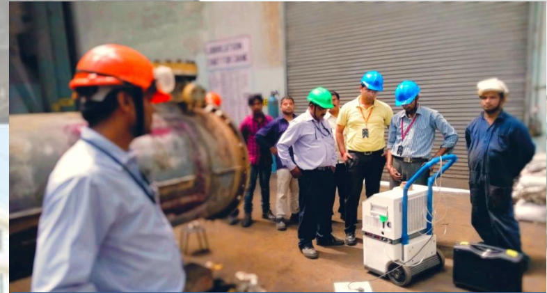
Helium Leak Testing of Heat Exchanger being done
