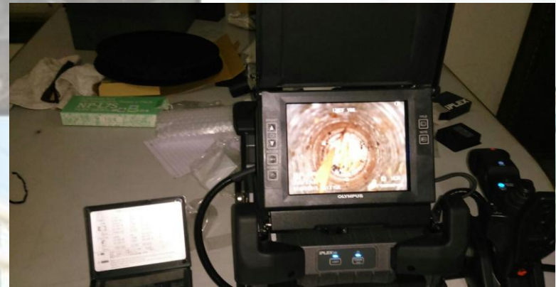
ITE's Industrial Borescope with 18 meter length and 6 mm dia.
