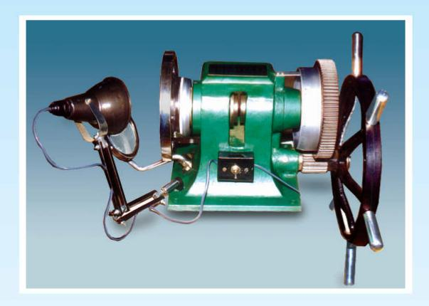
FIE Erichsen Tester is designed to carry out Erichsen Cupping Test on metals. Quick clamping and manual operation facilitates faster and trouble free working of the machine.
