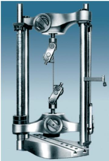
**ATTACHMENT FOR TENSION TEST FOR WIRE ROPES.**
