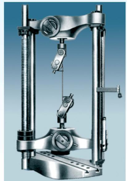
**Attachment for Tension Test for Wire Ropes**
