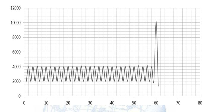
Cyclic and Load To Failure - Graph
