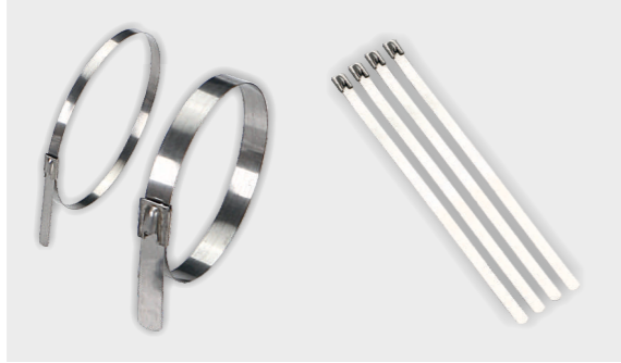
STAINLESS STEEL CABLE TIES (UN COATED) Ball - Self Locking Operating Temperature : - 80°C to 538°C Tensile Strength : 45 Kg.
