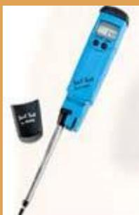
Lightweight and portable, this pocket tester directly measures soil conductivity and temperature. The penetration probe features a built-in temperature sensor, allowing for measurements that are automatically temperature compensated. The conductivity range can be calibrated at one point, and tester calibration is done in a standardized solution. Includes tester, 4.5"
