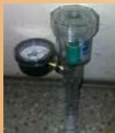
soil, it will allow water to flow freely through it, but not air. Tensiometer is available in standard lengths of 15, 30, 45, 60, 90, 120 cm. General use with row, tree, and field crops. Includes reservoir, air free gauge chamber, and hermetically sealed dial type vacuum gauge with dual
