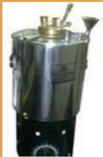
This apparatus is suitable for determining the close cup flash point of petroleum and mixtures according to IP-33 and IP-170 and also IS 1448 (Part-I) 1985. It is suitable for oils whose flashes below 70°C. It is supplied with oil cup cover fitted with stirrer thermometer socket S.S. water bath stand. An electric heater is fitted to bottom for operation on 220vAC circuits.
