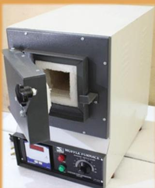
Light weight with ceramic fiber wool insulation (Instead of brick insulation). The distinct feature of perforated sheet is to prevent the temperature control unit from very high heat. Heating elements are made of KANTHAL A1 wire of coil form embedded on the muffle with high grade refractory cement and backed by high temperature cer-
