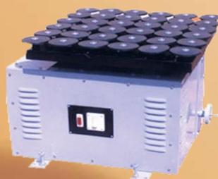
Compact bench type model with platform fitted with rubber dics, mounted in ball bearing crank shafts to give an orbital motion to the flask. The motor is coupled by means of V - belt with
