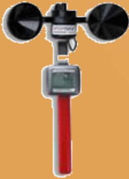
This Instrument comes with dual digital display measures speeds from 5 mph to over 125 mph. the unique tilting head fold flat for store. Water resistant display can be used in heavy rain. Multi-function display, in mph/h. Display current speed plus Average or max speed at the same time. Comfortable viny handle.3 cup rotor does not care which way the unit is pointed (unlike those little
