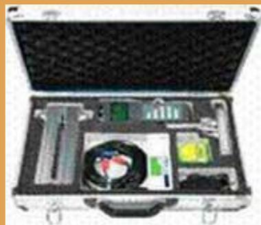
Portable ultrasonic flow meter that measures flow rate by calculating the spread time of ultrasonic water in fluids. The product is appreciated for its robust construction, accurate results, trouble free performance, negligible maintenance and much
