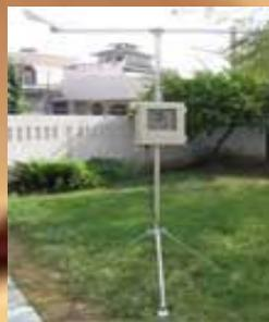
This is a micro controller based automatic wind monitor reflect state of the art in micro controller based instrumentation design. Both wind speed and direction sensors can be attached with this data logger for the collection of real time data automatically.
