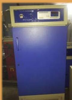
Double walled chamber with interior walls made of S.Steel. The exterior is made heavy mild steel finished with stoving white enamel. The door is also a double walled construction. The temperature range is from 5 - 60 Degree C, with an accuracy of +/-0.5 Degree C, controlled by Digital temperature controller cum indicator. Temperature
