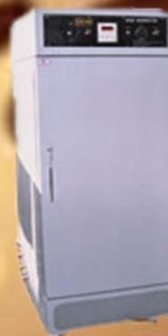
Doubled walled chamber with interior walls made of anodized S.Steel. The exterior is made of heavy mild steel finished with stoving white enamel. The temperature is controlled by Digital temperature controller cum indicator from ambient +5 - 50 Degree C , +/-2 Degree C and humidity from 60 - 95 % , +/-3%
