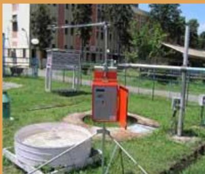
Kaizen make Digital Solar Radition Recorder is a self contained fully automatic solar data recorder fitted with solar panel & SLA battery based power system, High accuracy V-Log Data Logger & Power management system contained in a single IP65 waterproof fenclouser.
