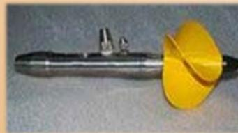
Universal Water Current Meter delivers for conviction of current velocities in water courses, canals, rivers and the sea. The equipment wallet will be vigorous interpretation made of Aluminum with locking arrangements. Velocity Range: 0.04 m/s ~ 10 m/s, Meter Material high Quality non-corrosive Brass is being used in body.
