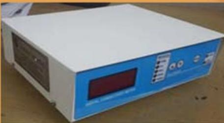
It consists of TDS and manageable temperature compensation to maintain accuracy. It has a function of automatic power
