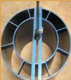
The double ring Infiltrometer is a simple instrument which is used to determine the infiltration rate of water into the soil. The infiltration rate is determined as the amount of water per surface area and time unit, which penetrates the soil. This rate can be calculated on the basis of the measurements and the
