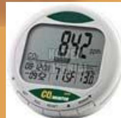
Max/Min CO2 value recall function, Visible and Audible CO2 warning alarm with relay output for ventilation control, Maintenance free NDIR CO2 sensor are some of the attributes you will notice in our Carbon Dioxide Monitor.
