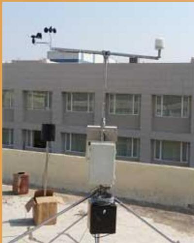
Kaizen make automatic weather station is a self contained fully automatic weather data recorder fitted with solar panel & SLA battery based power system, multi- channel high accuracy data logger with power management system contained in a single IP65 waterproof enclosure.
