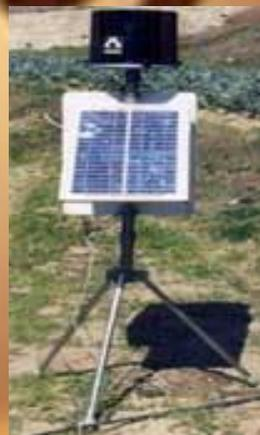
**KAIZEN IMPERIAL** make digital rainfall recorder is a self contained fully automatic rainfall data recorder fitted with solar panel & SLA battery based power system, High accuracy V Log Data Logger, GSM/GPRS based telemetric modern & power management system contained in a single IP65 waterproof enclosure.
