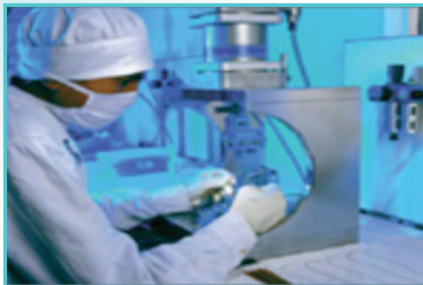
Needle crimping on a pneumatically operated crimping machine where eyeless needles are attached to individual suture strands
