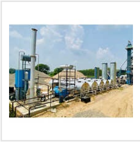
Indirect Heating Bitumen Tanks
