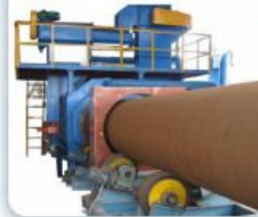
PIPE CLEANING SHOT BLASTING MACHINE
