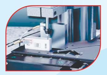
GAUGE BLOCK COMPARATOR (WITH TESA PROBES - TT-80)
