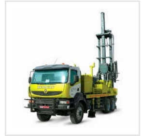
KLR KPR 5-42 Piling Pole Drill Rig
