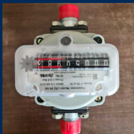
Commercial Gas Meter
