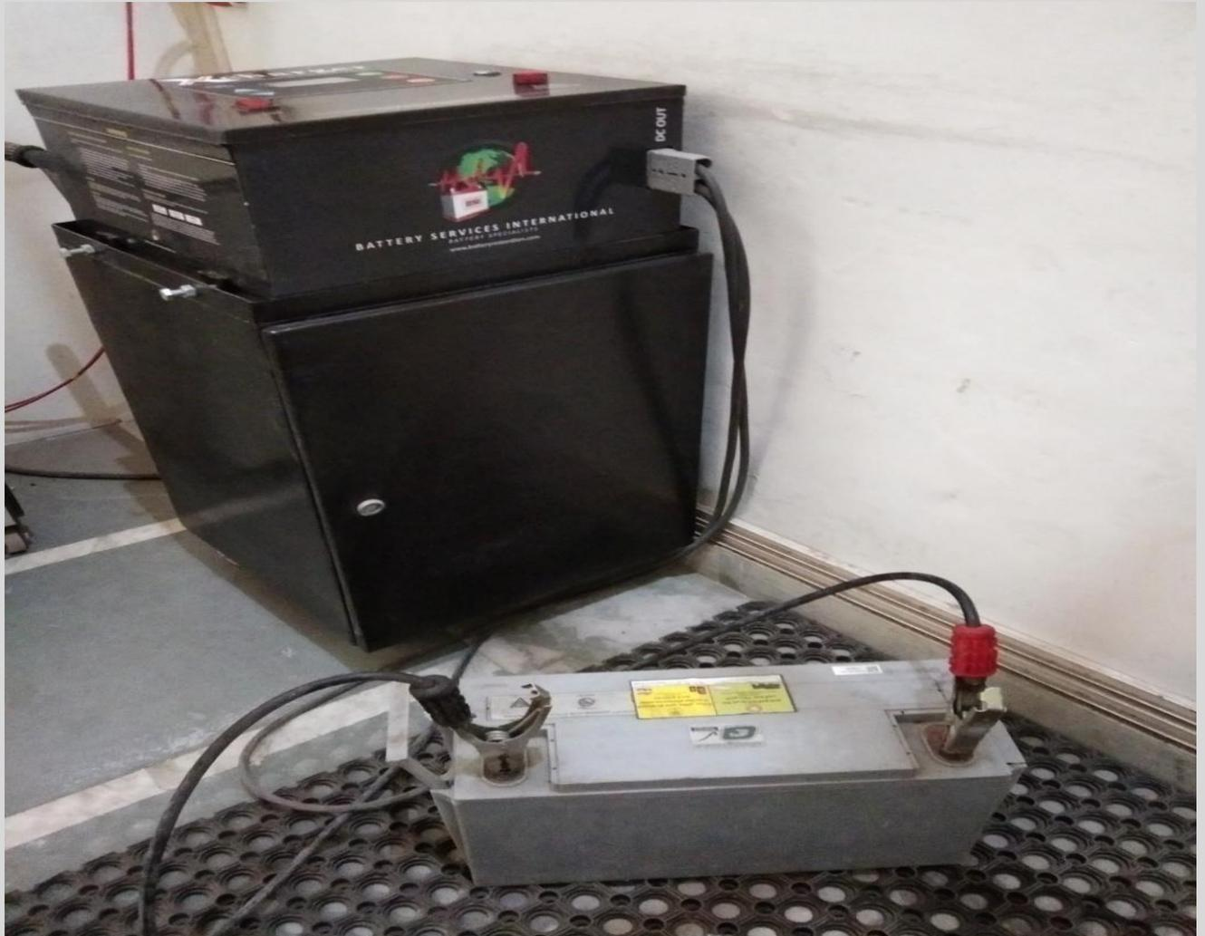
**Recovery and Charging:-** This function is designed to desulphate and recover the lost capacity of all types of lead acid batteries. The combination of charger and solution restores five potency in the battery and make it healthy. These potency are - **Voltage, Internal Resistance, Capacity, SOC and CCA.**
