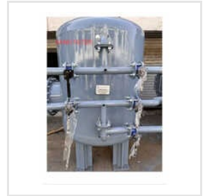
Pressure Sand Filters
