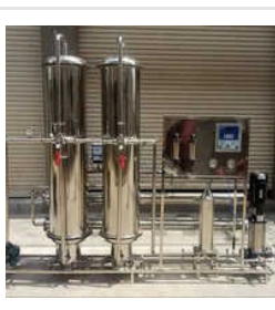
Reverse Osmosis Plants
