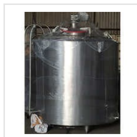
Vertical Milk Storage Tank
