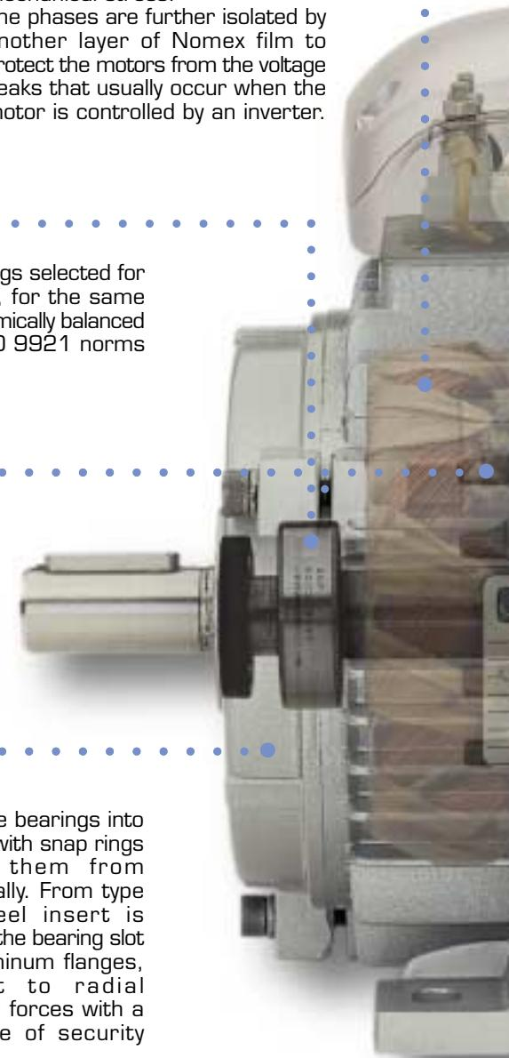
Blocking the bearings into their slots with snap rings prevents them from moving axially. From type 90, a steel insert is provided in the bearing slot of the aluminum flanges, to resist to radial mechanical forces with a fair degree of security
