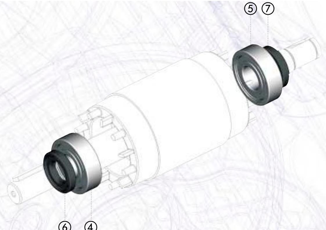
2 bearings lubrication devices on the front and the back shield are provided in motors from size 180 and up.
