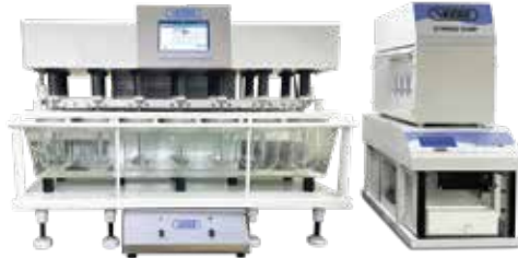
VDA-14D (T)+ VAS- S14 14-Station Dissolution Test App with Touchscreen Auto sampler with syringe pump
