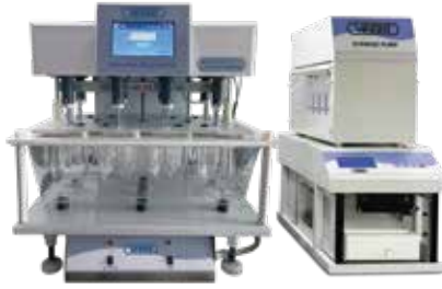
VDA-8D (T)+ VAS- S8 8-Station Dissolution Test App with Touchscreen Auto sampler with syringe pump
