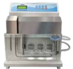
VTS-P Tablet Disintegration App for Pessaries & Suppositories
