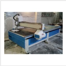
1530 Series Fully Automatic CNC Router
