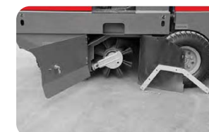
Rear brush provides maximum sweeping power against heavy debris
