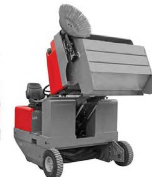
Hopper can be raised at heights up to 1.5 metres
