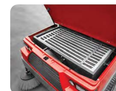
14 m² filtering surface with correct dust and air passage space between each element.
