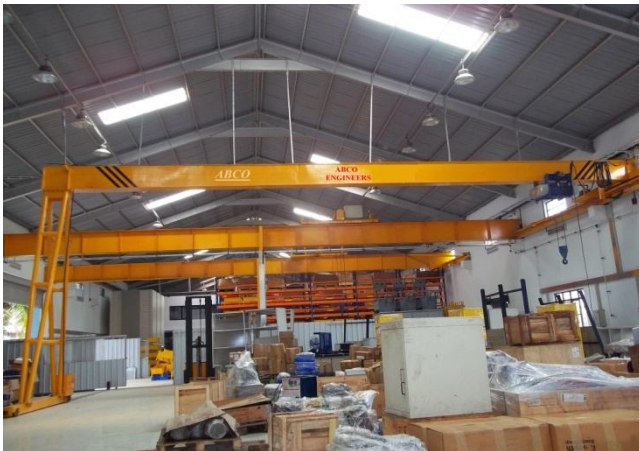
Customer: Bosch Rexroth, Bangalore 3 Ton Single Box Girder Semi Gantry Crane
