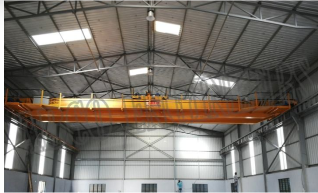
Customer: RamKorp Steel Tech Pvt. Ltd. Bangalore 10 Ton Single Girder EOT Crane
