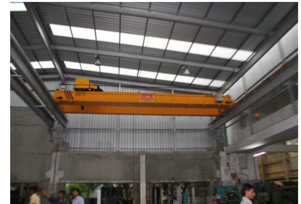
Customer: Prabha Industries . Bangalore 7.5/3T Double Box Girder EOT Crane. (In Association with THAC, Taiwan)
