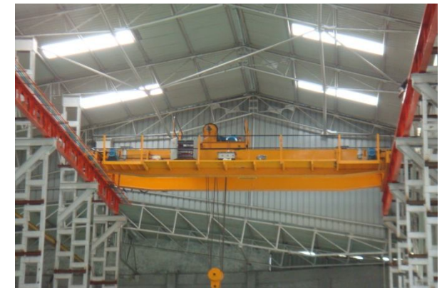
Customer: Universal Power Transformers, Haridwar 20Ton Double Box Girder EOT Crane. (
