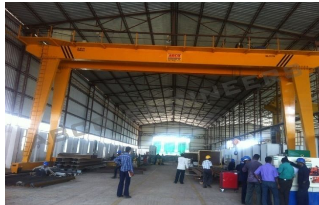
Customer: CAMFIL FARRA Air Filtration India P. LTD 15/3Ton Double Box Girder Goliath Crane(Trichy)
