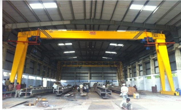
Customer: Baby Engineering Private Ltd. Trichy 10+10 Ton Single Girder Gantry Crane
