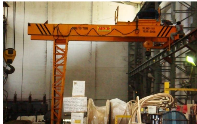
Customer: Universal Power Transformers 10 Ton Double Box Girder Semi-Gantry Crane
