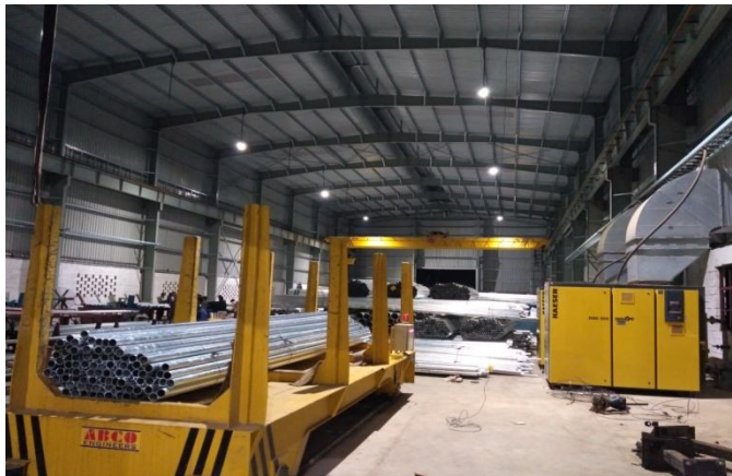
Customer: SURYA Roshni Limited, Hindupur 10 Ton Capacity Pipe Transfer Car
