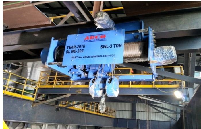
Customer: JSW Steel Limited 3Ton x 12M HOL Electric Wire Rope Hoist
