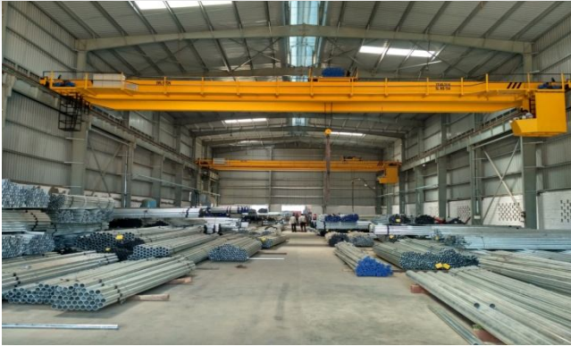
Customer: SURYA Roshni Limited, Hindupur 5 Ton Double Box Girder EOT Crane
