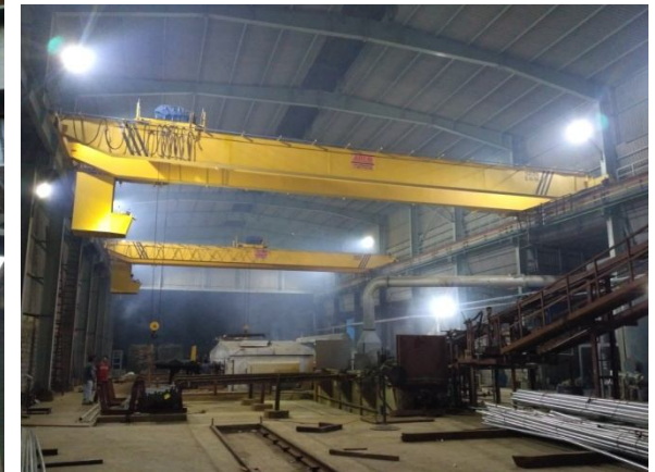
Customer: SURYA Roshni Limited, Hindupur 5Ton Double Box Girder EOT Crane
