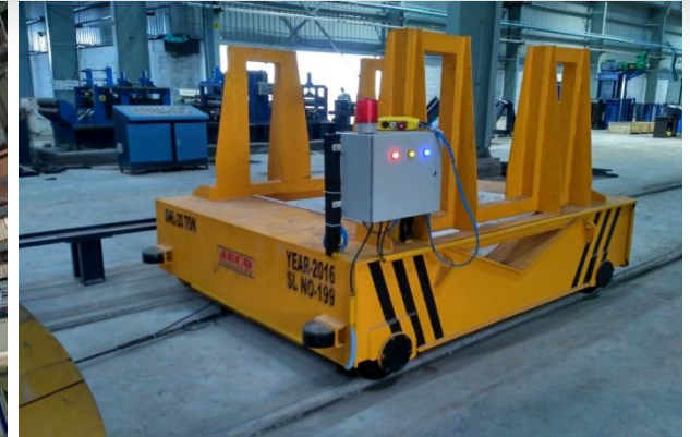
Customer: SURYA Roshni Limited, Hindupur 20Ton Capacity Coil Transfer Car
