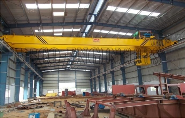
Customer: APL APOLLO Tubes Pvt. Ltd. Hosur 10Ton Double Box Girder EOT Crane
