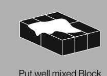
Put well mixed Block Jointing on the block with help uniformly on the unit for a min 4mm bed thickness.
