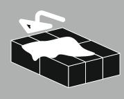
Block Jointing to be applied on block and on column for good bonding of the joints.
