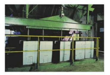
Calibration System: Built-in certified test weights allow testing from the control room assuring accuracy in weighing performance for every train.
