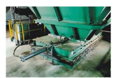
**Dustless Control Gates:** Double-blade Slide-gate design allows for quick response to control signals for the accurate cut-off assuring consistent weight wagon after wagon.
