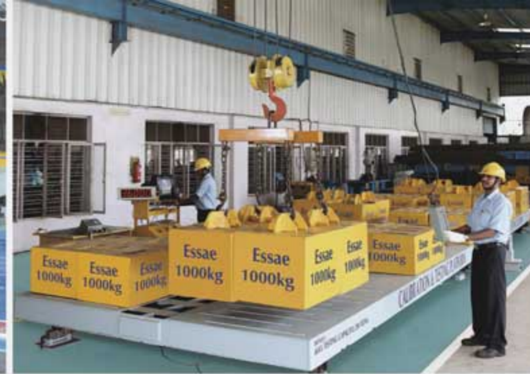
Full capacity Calibration Testing of Load Cells
