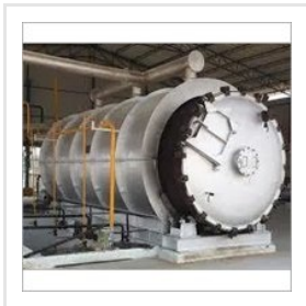
Waste Tire Pyrolysis Plant
