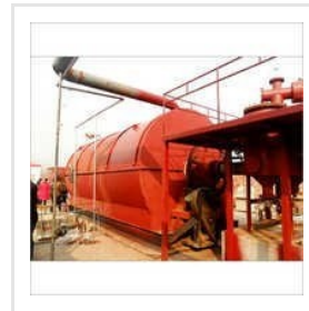
Rubber Tyre Recycling Plant
