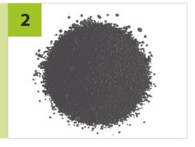
**Scrap Steel (13-15%):** Scrap Steel is the third high-value byproduct of the pyrolysis process, derived from the steel beads found in radial tires. Pyrolysis steel has a good market demand, The scrap steel is sold to rolling mills as raw material, where it is transformed into valuable products by further processing.
