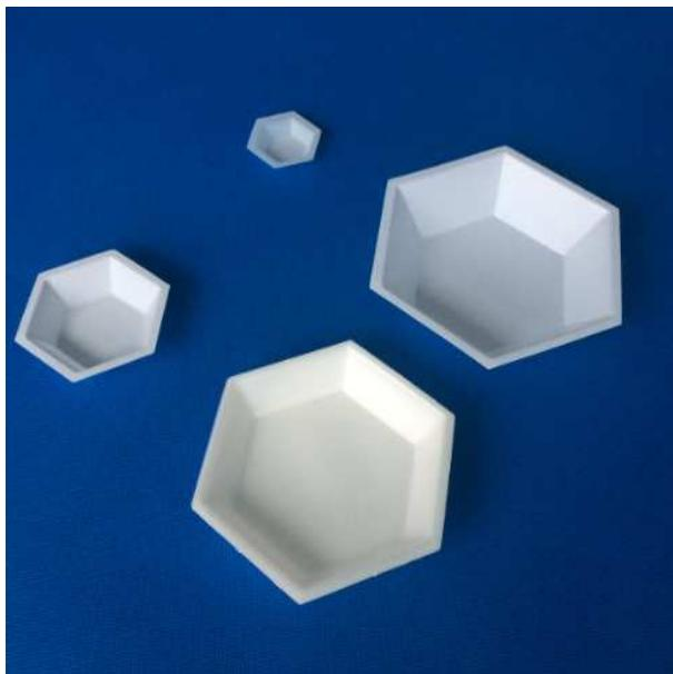
Disposable Weighing Dishes/Boats can be utilized for liquid or solid balance sample during weighing procedures. The smooth surface and rounded corners provide for easy removal of powdered and granular samples. Polystyrene materials flexes to allow bending of the weighing boats.
