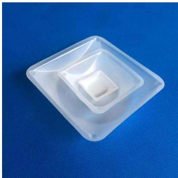
Disposable Weighing Dishes/Boats can be utilized for liquid or solid balance sample during weighing procedures. The smooth surface and rounded corners provide for easy removal of powdered and granular samples. Polystyrene materials flexes to allow bending of the weighing boats. Recesses at the corners facilitate controlled pour-off.
