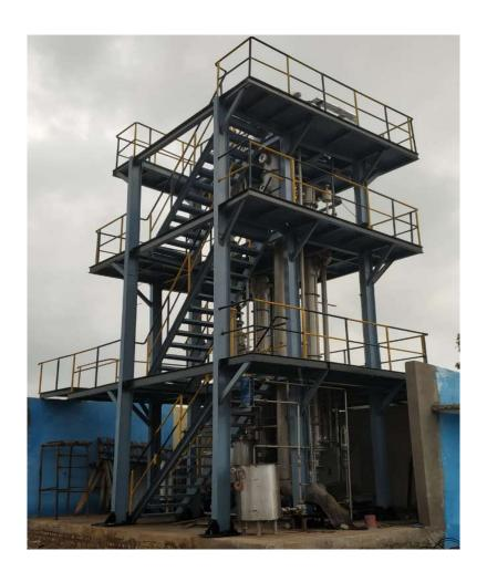
KEP Engineering has completed the manufacture and execution of Skid mounted 15KLPD of Zero Liquid Discharge system. For this we have supplied for Double Effect Evaporator followed by Agitated Thin Film Dryer. KEP strive to serve for 100% client satisfaction by deputy qualified engineering. Efforts from all corners of KEP made us to complete this project successfully with zero errors.
