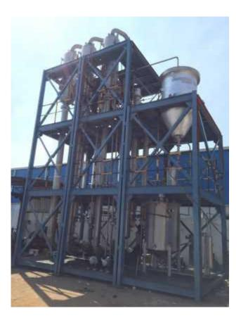
KEP Engineering has completed the manufacturing and execution of Skid mounted 40 KLPD. For this we have supplied for Triple Effect Evaporator followed by Pusher Centrifuge. In inhouse we have run the plant with pusher centrifuge it is successfully executed this is only because good efforts. KEP strive to serve for 100% client satisfaction by deputy qualified engineering.
