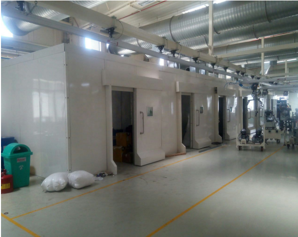
Acoustic Chamber for Two Wheeler Engine Noise Testing
