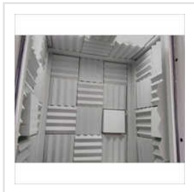
Test Lab Acoustic Enclosure
