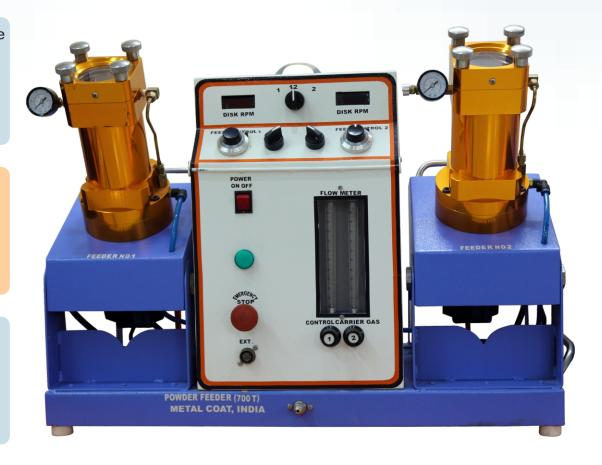
The MPF 700 Twin Powder Feeder is specifically designed for thermal spray coatings. Its small size makes it a portable powder feeder, which can be carried to site for job work. The unit is controlled to extremely precise and repeatable feed rates. The powder hopper (canister) is mounted on a
