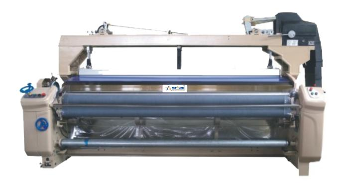
This series designed, based on heavy water jet loom, which is optimizing the main component and frame structure improving the beating – up, let-off mechanism and take up mechanism, installing assistant device on let-off mechanism, all of the ensure the running stability and reduced the vibration and noise, increased efficiency and enlarged the weaving range.
