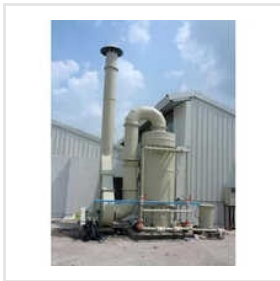
Industrial FRP Scrubber
