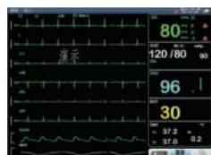
Max 8 waveform display simultaneously, max 6 leads ECG waveforms display
