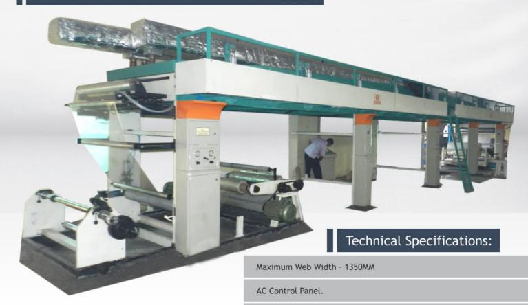
Speed: - 35 meter/ min. (The operating speed is usually influenced by the type and
