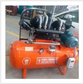
10HP Triple Cylinder Compressor
