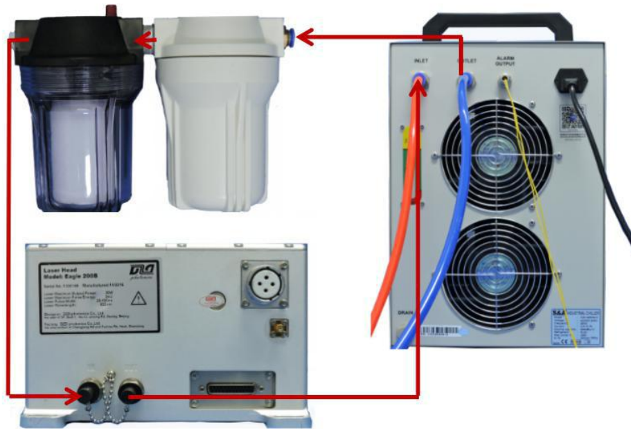
Fig.2-7 Cooling water circulation direction
