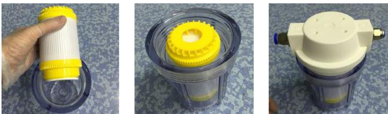
Fig.6-2 Steps of replacing the Deionized filter
