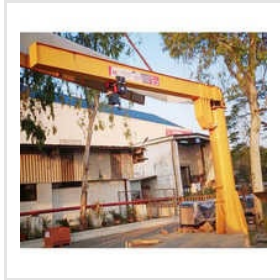
Tower Pillar Mounted Jib Crane
