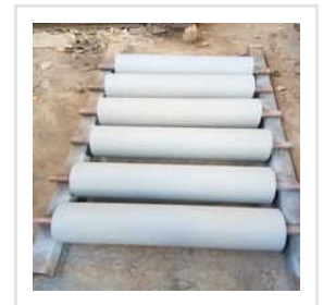
Belt Conveyor Head Pulley
