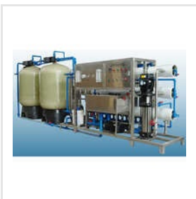
Water RO Plant
